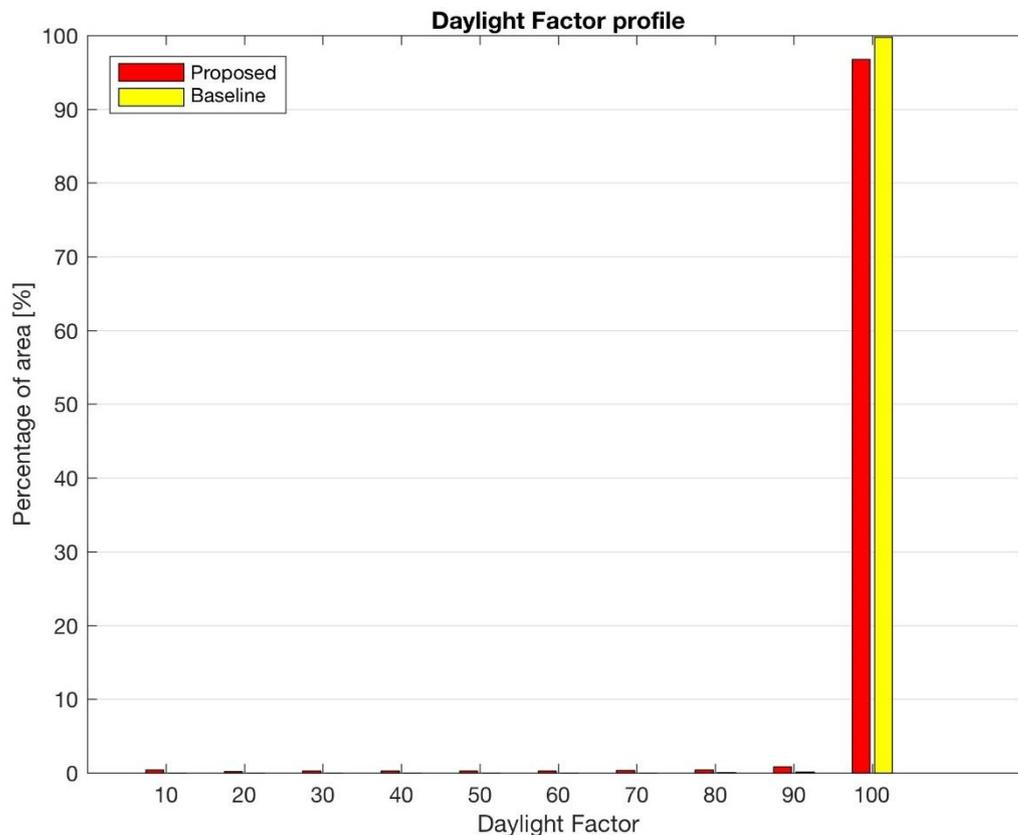
The area receiving a certain daylight factor value is represented by the length of the corresponding bar. The baseline is receiving 100% daylight factor for almost all its extent (99% percentage of area at 100% daylight factor). The proposed road development has a limited effect, reducing this area by approximately 3% (97% of the total area achieves a daylight factor of 100%).
