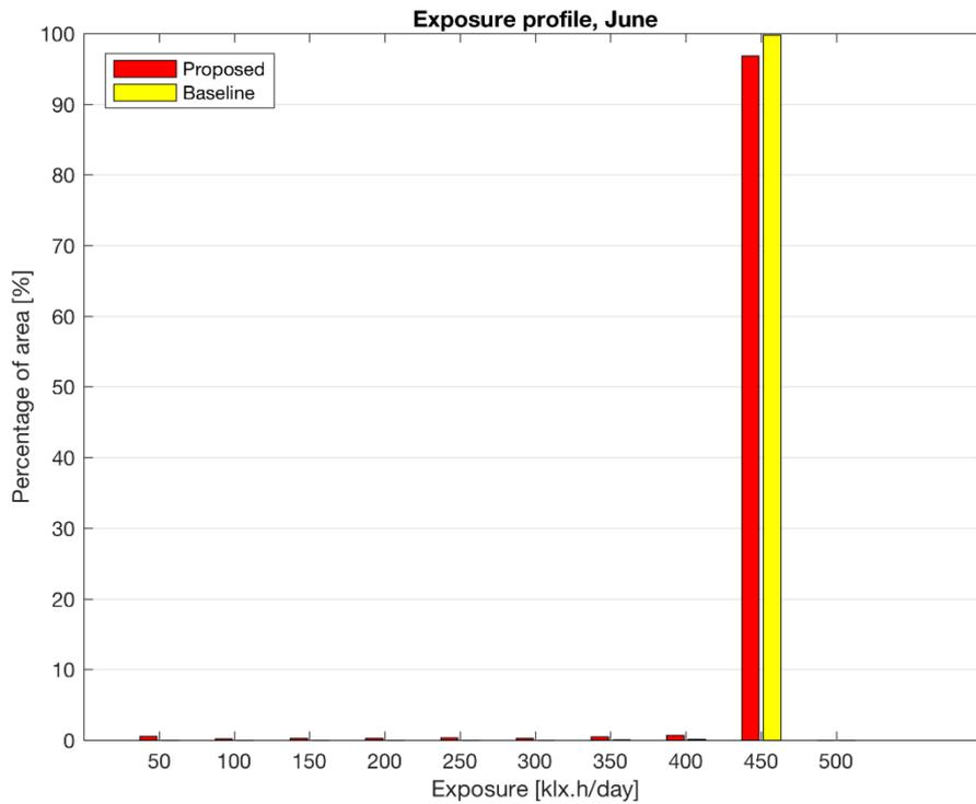
The chart shows the percentage of area within a certain exposure value. As it can be seen, for grid 2, the proposed condition has a reduction of area exposed to the maximum sunlight and daylight available of around 3%.
