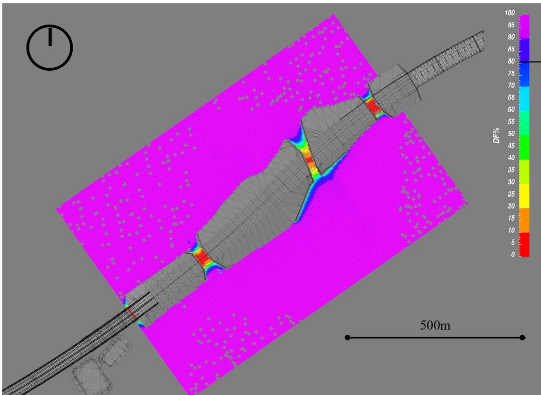
**Figure 14: Grid 2 daylight factor distribution, proposed road development. Note that grid 2 encompasses grid 3, 4 and 5**
