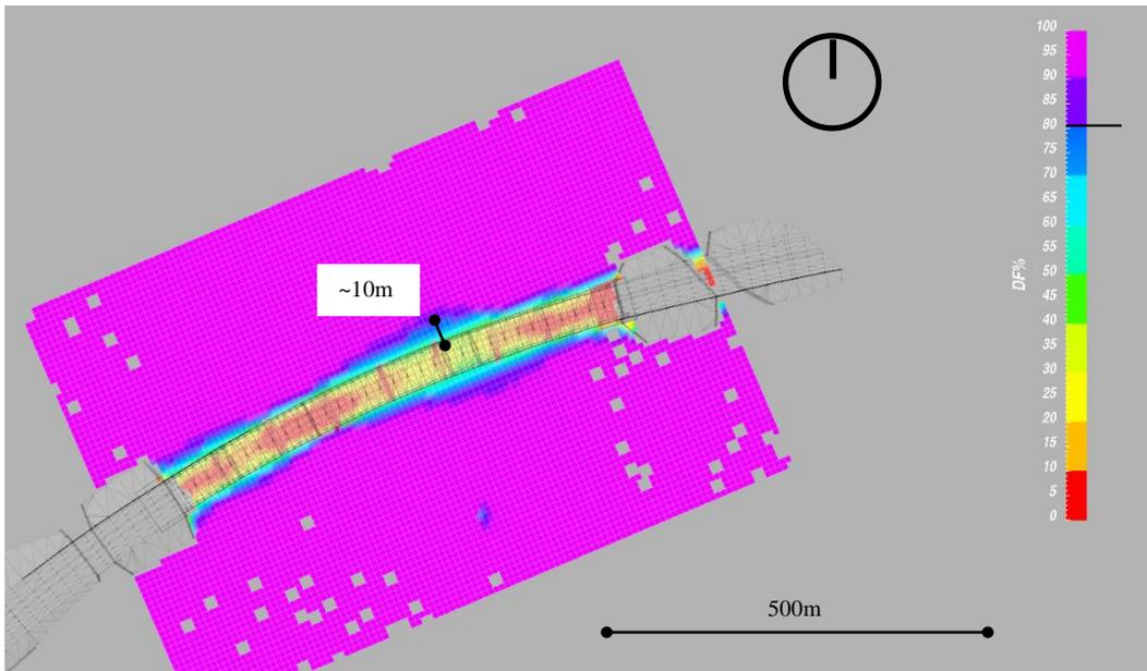
**Figure 12: Grid 4 daylight factor distribution, proposed road development**
