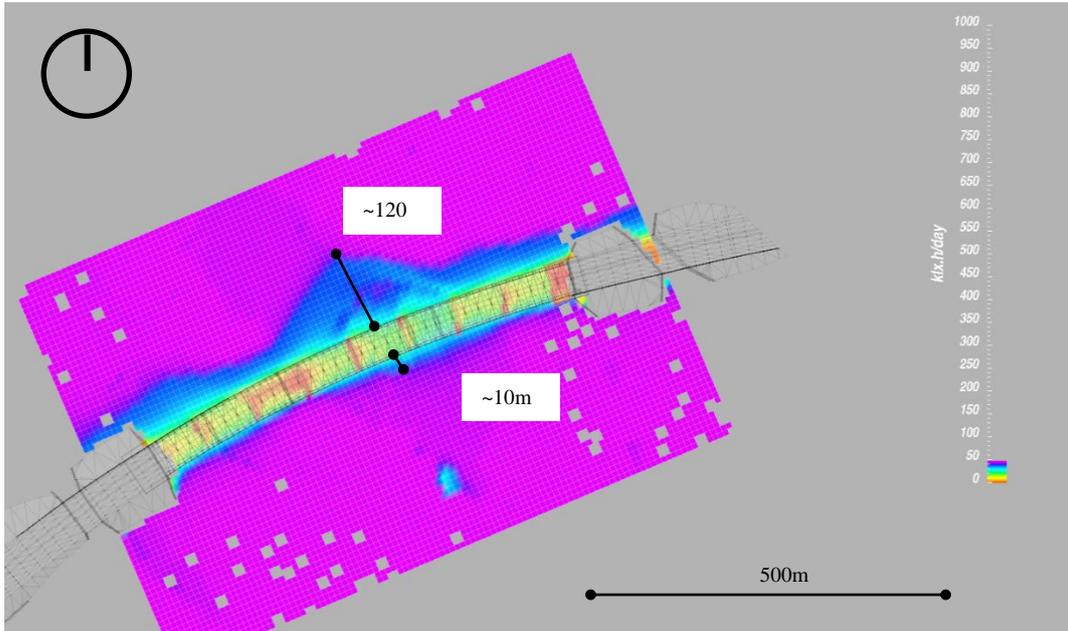
**Figure 16: Daylight average daily exposure for June at grid 3**
